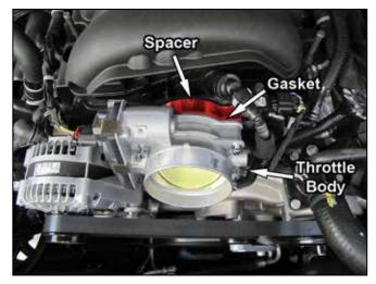
5. Install the provided new bolts through the holes in the throttle body, through the holes in the provided gasket and through the POWERAID spacer. Start the new bolts into the inserts in the intake manifold being careful not to cross thread the bolts. Tighten the bolts in a cross pattern to the factory specifications. **NOTE: Be sure to install the spacer in the correct direction as noted on the spacer.**
